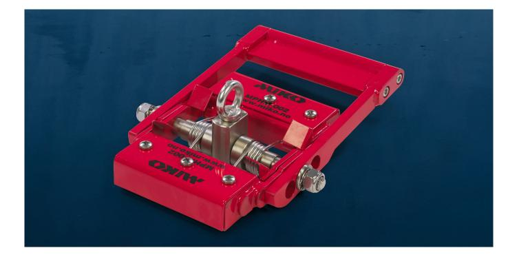
The magnetic component consists of neodymium which is coated with epoxy to improve its corrosion resistance in sea water. With a holding force of 150 kg, the magnet can be used for fastening diving equipment, guide wires or anchor points for divers to pipes or other cylindrical steel structures.
